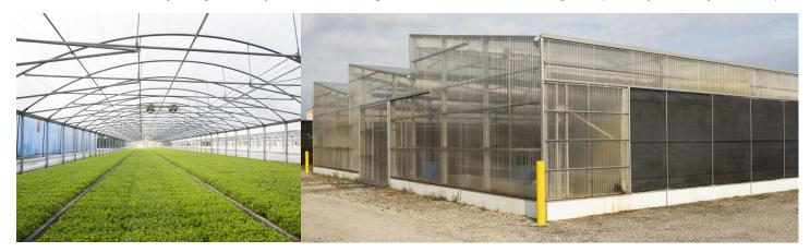
**Shade houses** can vary in construction, but are often a metal structure covered with black mesh/shade cloth to limit light and UV exposure. Most are not categorized as a building, but still possess the same safety concerns.
